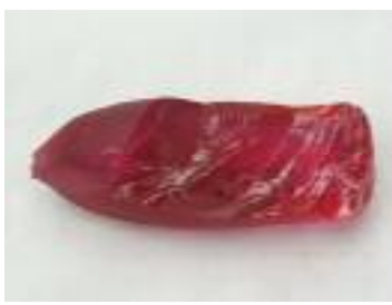
Synthetic Ruby by Verneuil Process
